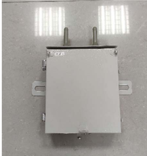
Figure 4 Illustration of Sub-transmitter (outdoor high-voltage PT power supply; PT output voltage 220V)
